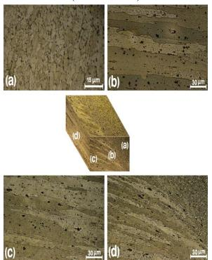
**Fig: 3.** Optical micrographs of different zones of FSP sample: (a) NZ, (b) TMAZ, (c) HAZ, and (d) BM (B. Zahmatkesh<sup>8</sup>)
