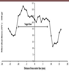
Fig: 4. Micro-hardness profile measured on the cross section of the FSP zone B. Zahmatkesh <sup>8</sup>
